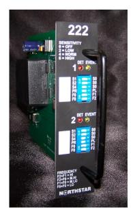
The N222 has been specifically designed and engineered for use in the demanding Traffic Control industry. With standard operations including: seven sensitivities, four frequencies and selectable presence time options. The N222 covers your detection needs.
