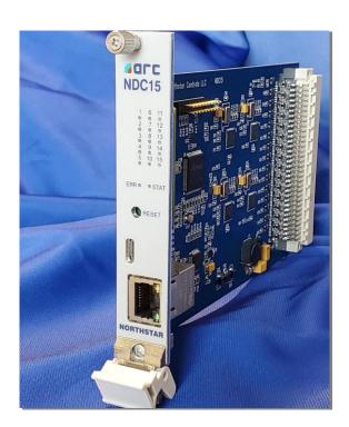
The NDC4 /15 serial data modules are intended to collect data streams from individual detectors in a compatible card rack and transmit the data in packet form to a host for use in an AVC system.
