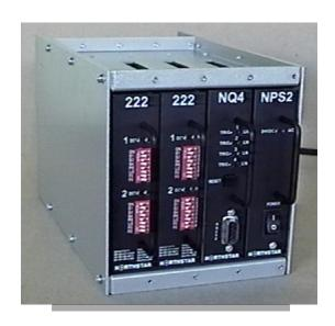
The NQ4 has been specifically designed and engineered for use in special application traffic control and warning situations such as: Over speed/Over length detection, truck roll over advisory and blind curve warning. Information the user may view via laptop computer connected to the front panel DB9 of the NQ4's Logic Module include: current set-up, and current data such as speed, length and lane.
