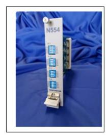
The N554 has been specifically designed to provide axle detection for use in vehicle classification systems for the tolling industry. The data provided by the N224-iS enables the latest algorithms to develop highly accurate vehicle classification.
